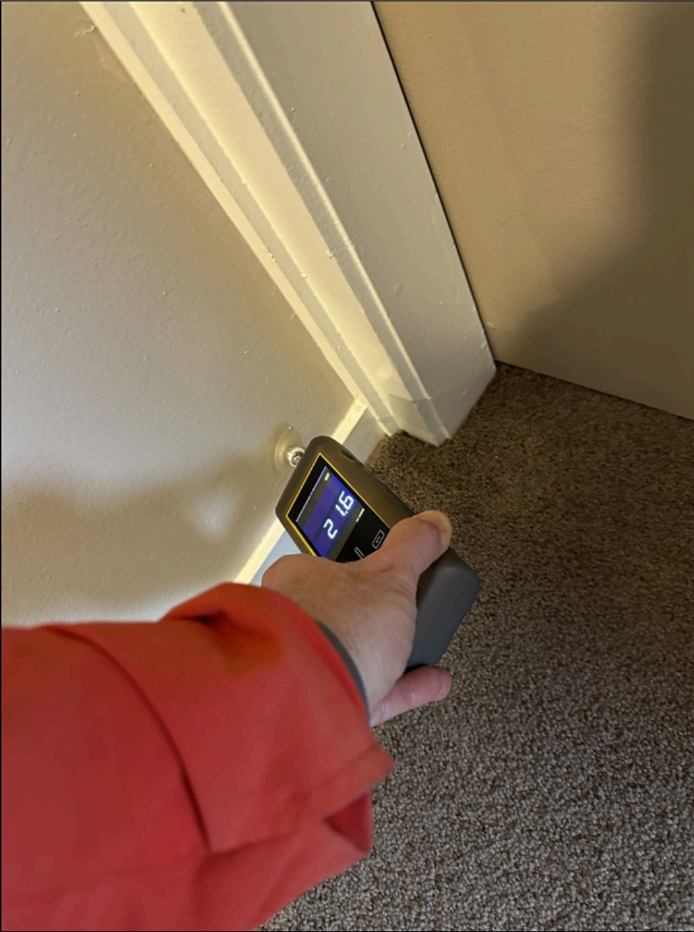
5.19.F Item 7(Picture) All Moisture Levels Within The Dry Range When Tested
