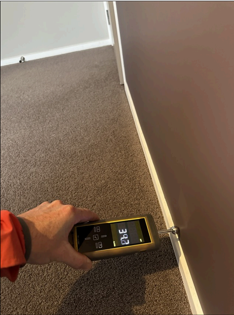
5.19.F Item 3(Picture) All Moisture Levels Within The Dry Range When Tested
