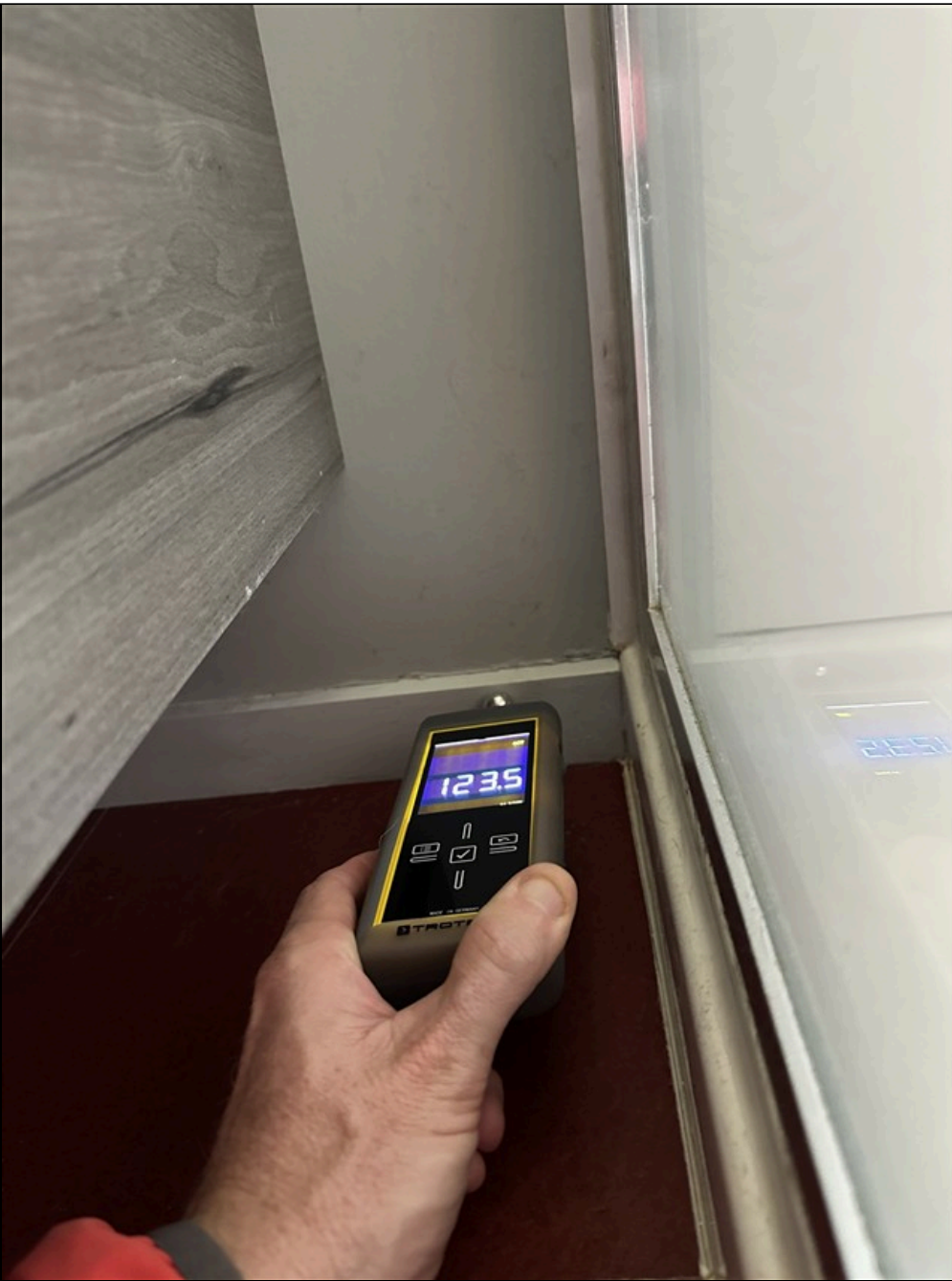
5.19.F Item 13(Picture) Some Signs Of Moisture In The Skirting Next To The Shower Unit
