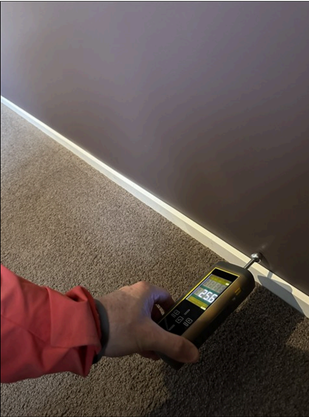
5.19.F Item 2(Picture) All Moisture Levels Within The Dry Range When Tested
