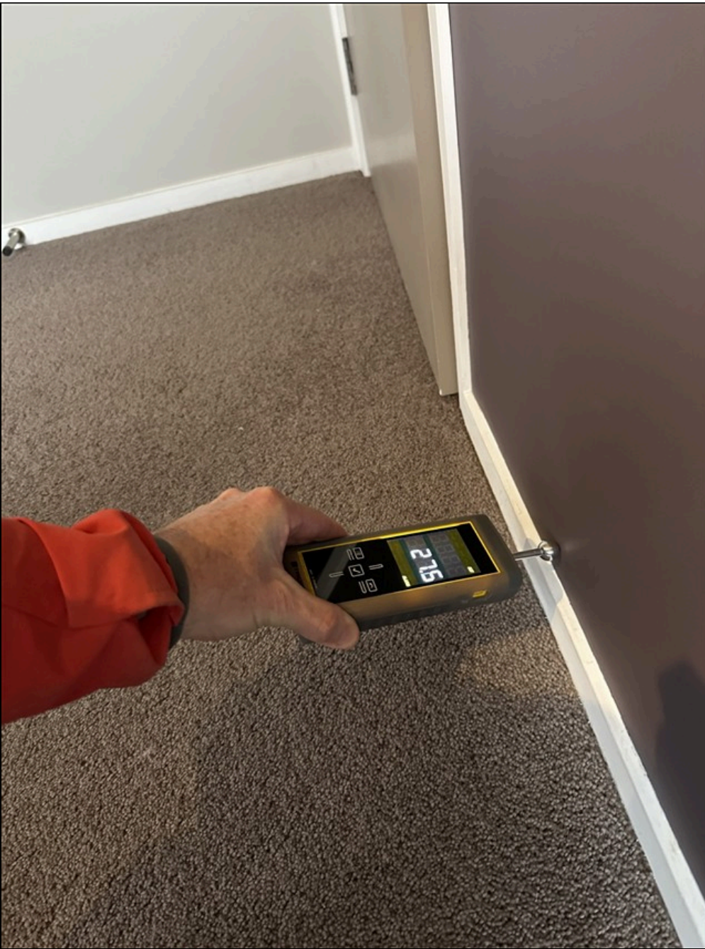
5.19.F Item 4(Picture) All Moisture Levels Within The Dry Range When Tested
