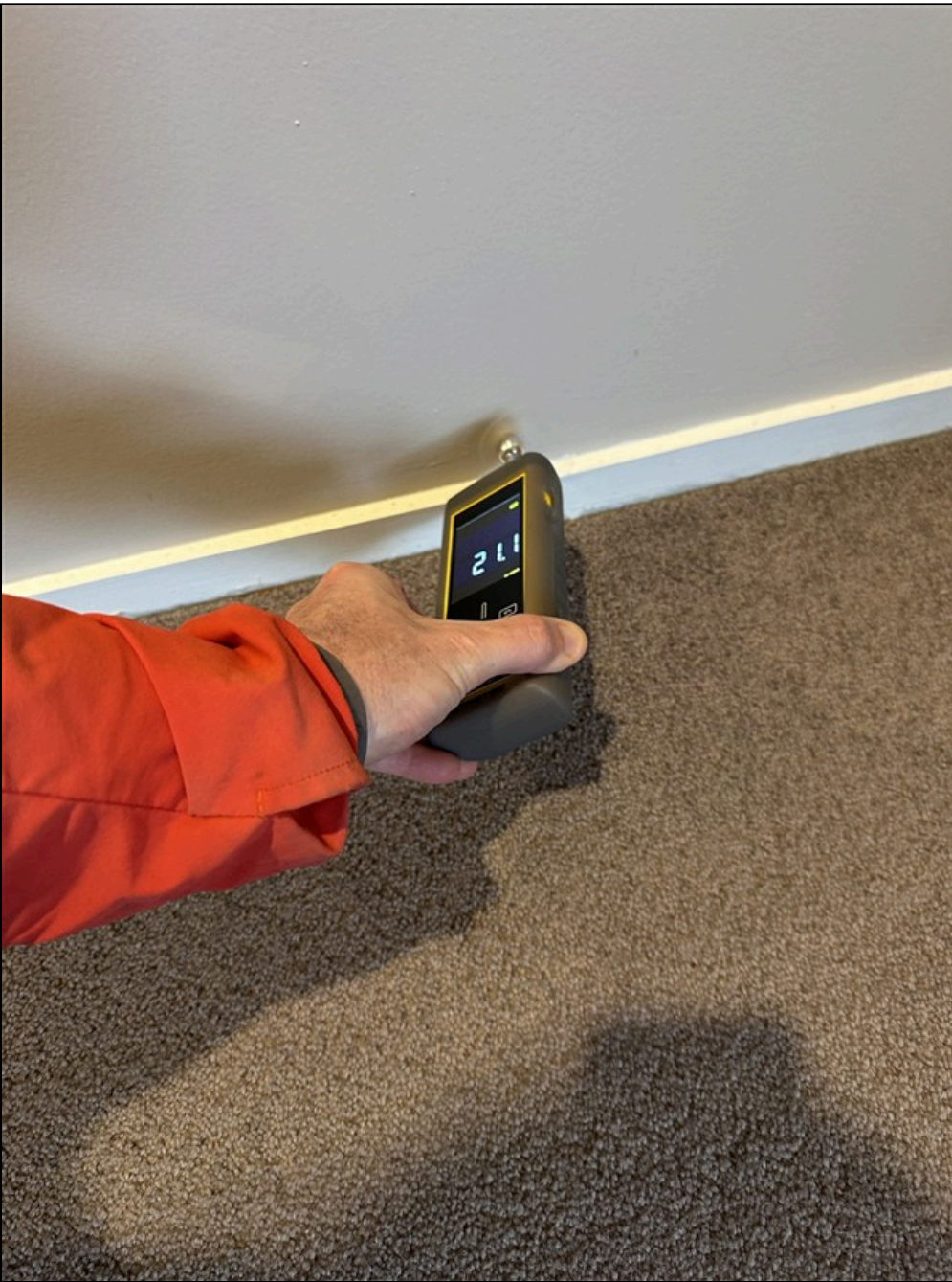
5.19.F Item 6(Picture) All Moisture Levels Within The Dry Range When Tested
