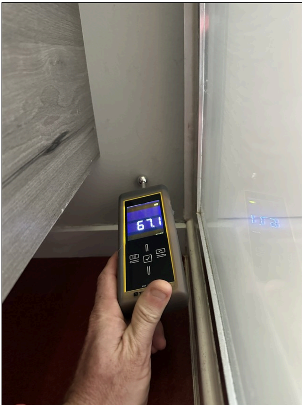
5.19.F Item 14(Picture) Some Signs Of Moisture In The Plasterboard Next To The Shower Unit
